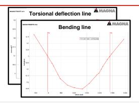
Global characteristics of a car body such as torsion, bending stiffness and other evaluations available.
