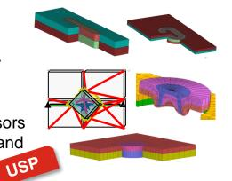
Identification of **stress conditions** of **spotwelds**, areas with **high deformation** in a **flange** based on several load cases in early project phases. **optimization** regarding number and position.
